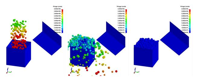
The next series of images shows the scraping process. The scraper moves across the top of the container leveling off any excess material.
