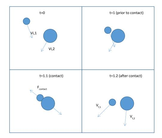
Motion (position, s and velocity, v) of particles is calculated in space for each time step:
