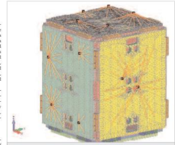
This is a satellite FEA model showing instrumentation attachment points (black squares) for isolated mass elements as defined by a center of gravity connected by rigid links (orange lines). The model is driven with an input power spectral density (PSD) function.
