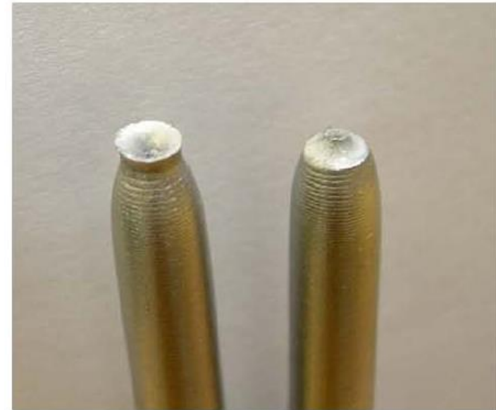
Figure 3. 'Cup and Cone' Type Failure
