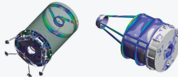
LS-DYNA TURBINE BURST SIMULATION
