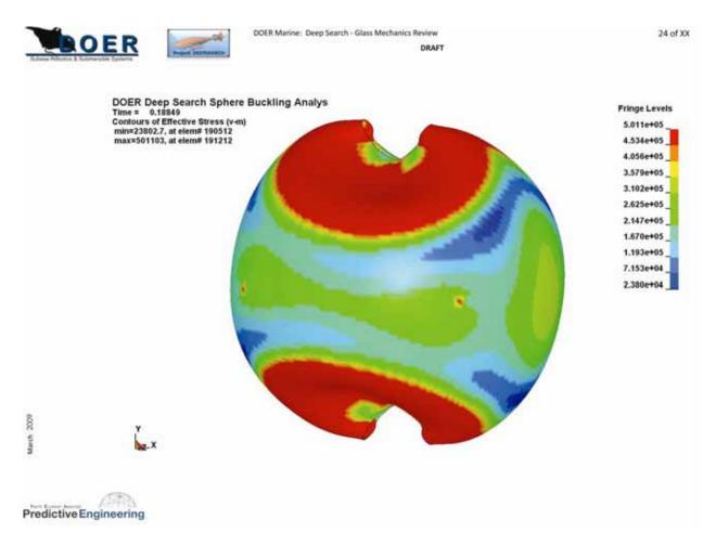
Early FEA study that indicates FoS of ~4X for bucking failure of the concept sphere.
