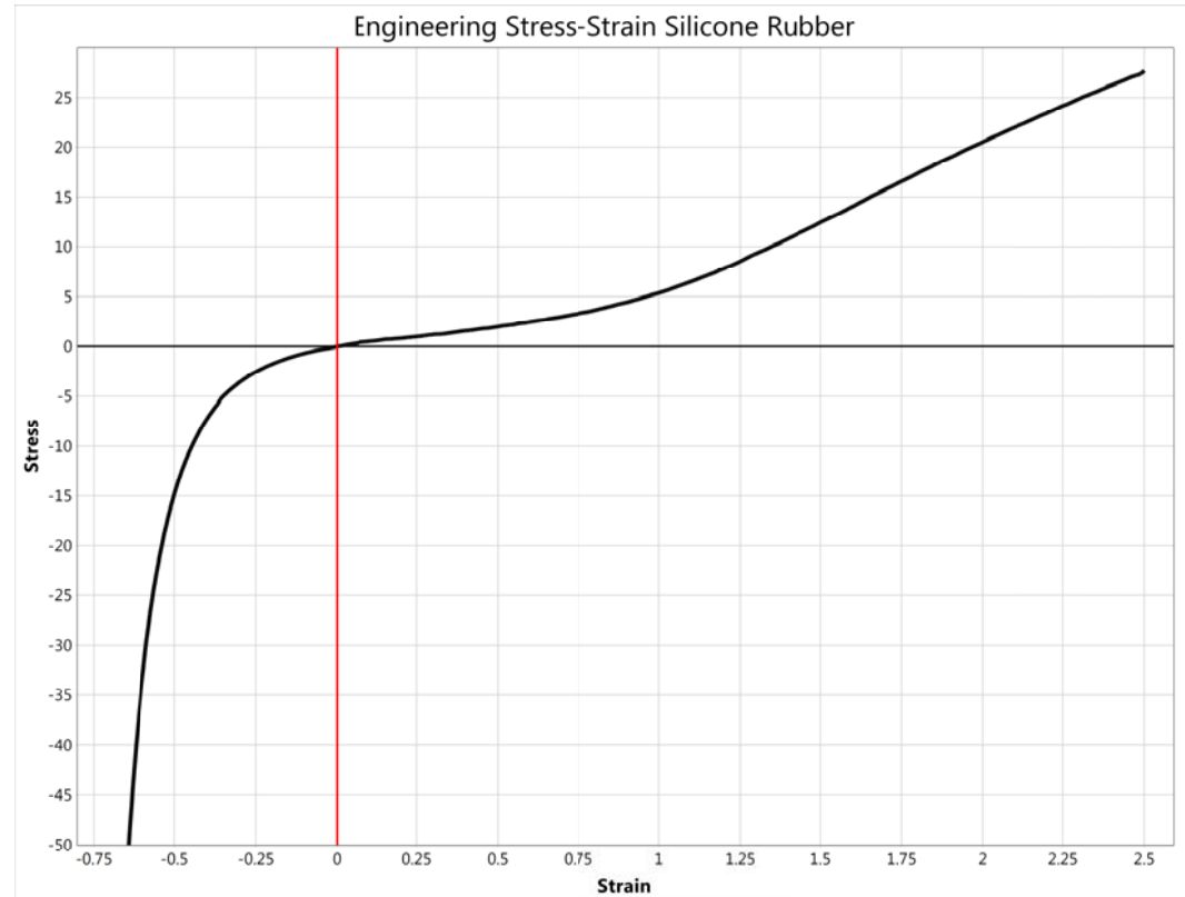
Figure 2: Classic Mooney-Rivlin idealization to the more accurate exact stress-strain formulation of *MAT_181
